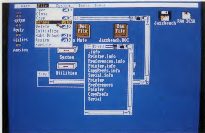
Hidden files can have default icons assigned to them with Jazzbench, so you can see everything that lies on a disk. Alternatively, you can view files in text format.
